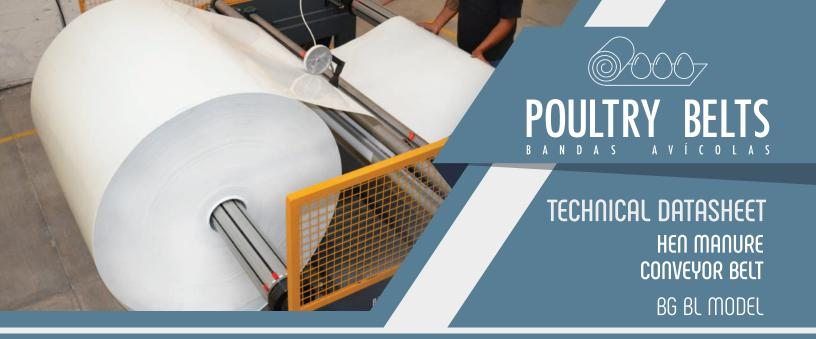
Our hen manure conveyor belts are manufactured from a high tenacity polypropylene copolymer, which offers greater resistance to elongation than other competing conveyor belts. Our products are also made of 100% high-quality virgin raw materials (LYONDELLBASSELL MOPLEN EP440G).
